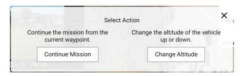
To continue from a specified waypoint, click on the desired waypoint via the QGC map to bring up the slider to Adjust current waypoint. Slide to confirm and press the Action button to bring up the Continue Mission slider to resume from the selected waypoint.
