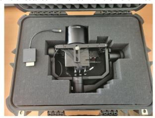
• Remove the rubber protector from the top of the gimbal. Looking down at the top of the gimbal, rotate the top of the gimbal until the white line and T3 symbol are facing forward (the direction of the camera lens).
