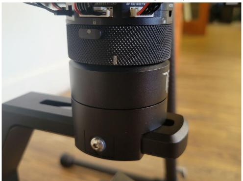
• Check to make sure all connections are securely plugged into the back of the camera and at the bottom of the gimbal below the camera.
