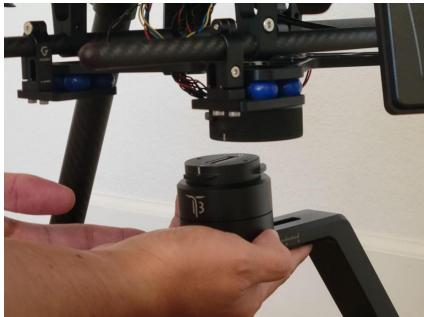
• Fully insert the gimbal to the quick connect mount and twist the drone side connection to the left to the lock position indicated by the lock symbol. The button will click into place and extend when the fully locked position is achieved.
