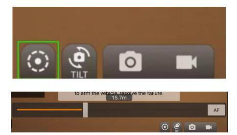
• To take a picture manually, use the MavCam photo trigger button. Photos will automatically be triggered during a mission.
