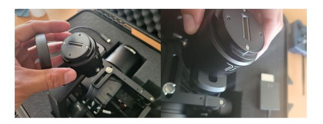
• With the gimbal centered, bring the payload to the front of the vehicle. The vehicle quick connect has a white line that will match up with the white line of the gimbal, make sure they both face towards the front of the vehicle when installing.
