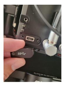
• With the vehicle and camera powered on, connect to the USB-C port using a computer with the iX Capture software. First select the settings tab, then the camera tab and scroll down until you see the Format Card option. It will only take a moment to format the card.
