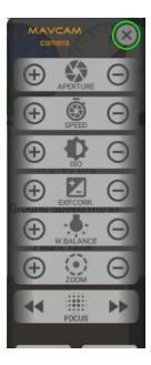
Under the swiped up MavCam settings, the C1 button is used to control auto camera settings. You will see under the Histogram on the left side of the screen the ISO, Aperture and Shutter Speed turn blue when auto settings are enabled.
