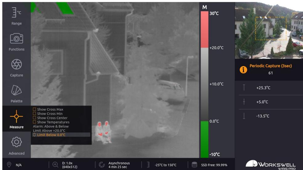
Figure 13.7: Alarm display – ABOVE & BELOW.
