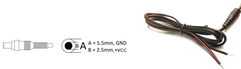
Figure 7.7: Inner power pinout, form of the common cable.
